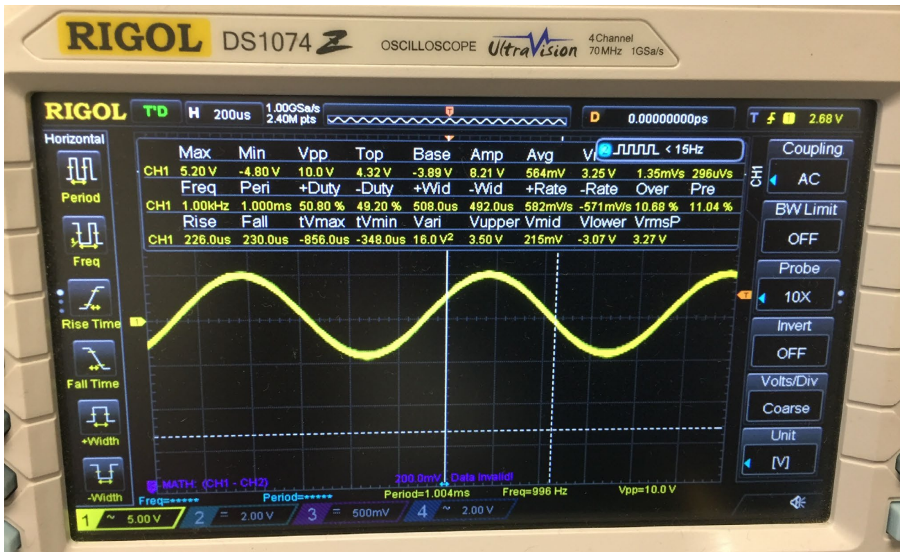
Figure 3.6: Photo of Rigol DS1074 Oscilloscope with a 10Vp-p sine wave at 1 kHz.
